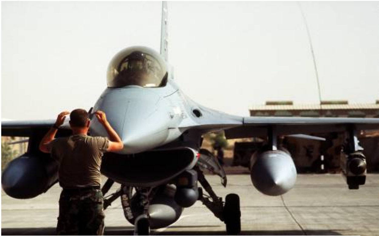
388th Tactical Fighter Wing F-16 with LANTIRN navigation pod mounted on the right side of the engine.
